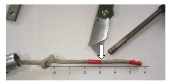
6. Cut rope at the edge of the tape, away from the knot.
