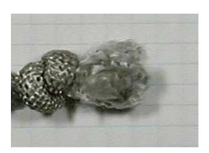
And this is how it looks when the glider tire rolls over the rope end.
