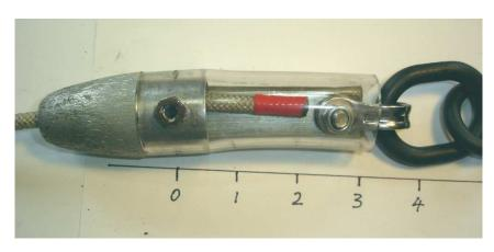
10. This shows the finished cable end piece assembly. The rope end will retract about ½" after the first tow. It is still easy to verify that the rope end has not been pulled to far in.
