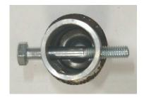
8. **NOTE**: The holes in the aluminum cable end piece and the clear plastic tube are "off center". This is necessary for correct mounting of the weak link assembly.
